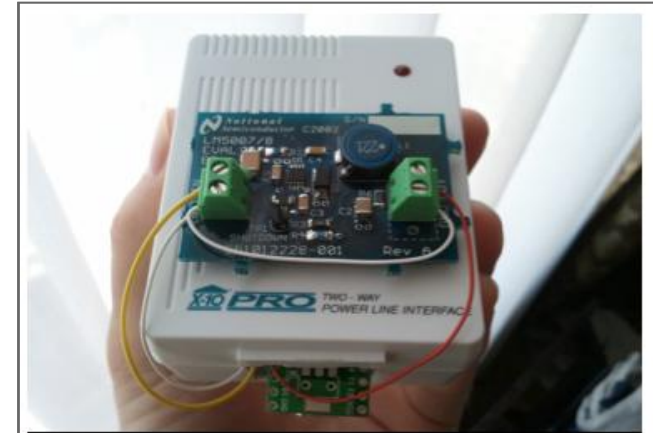
The X10 jammer designed by researchers to hack home automation systems through power lines. Photo courtesy of David Kennedy and Rob Simon.
